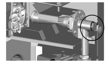
2. Without removing anything else, remove the nozzle from the burner inserting the screwdriver as indicated by the arrow.
